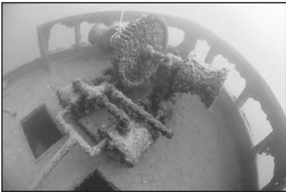
A windlass—a steam-powered device that hauled up the A.J. Goddard's anchor—was found, mostly intact, on the boat's stern in June 2009. The windlass was extremely large for such a relatively small boat, project leader Pollack said.
